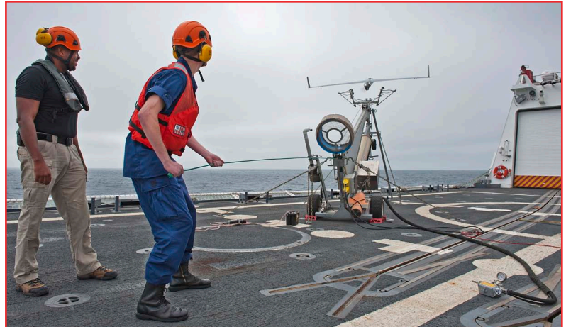
PACIFIC OCEAN – Petty Officer 3rd Class John Cartwright, a Coast Guard Cutter Stratton crewmember, releases the Unmanned Aircraft System ScanEagle during a demonstration approximately 150 miles off the Pacific Coast, Aug. 12, 2012. The ScanEagle is being demonstrated as a proof of concept for future deployments of small UAS aboard the National Security Cutter fleet. U.S. Coast Guard photo by Petty Officer 2nd Class Luke Clayton.
